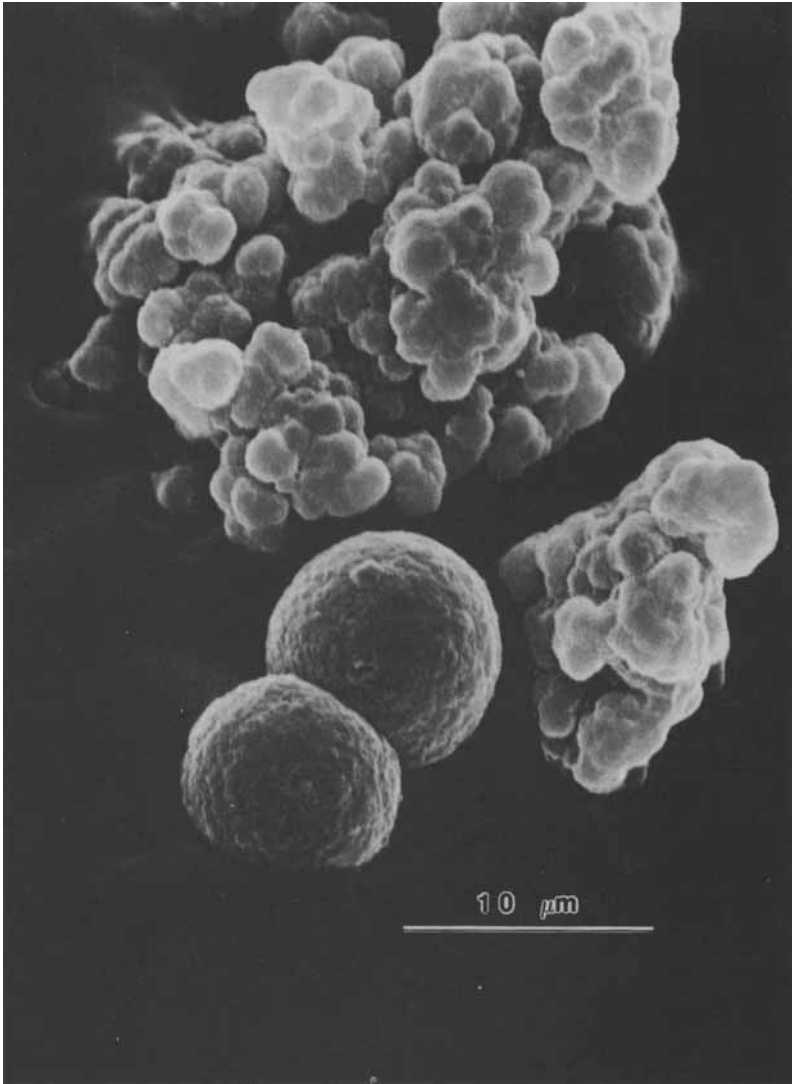
FIGURE 8d Scanning electron micrographs of particles obtained from dilute solution cures of UF resins.
