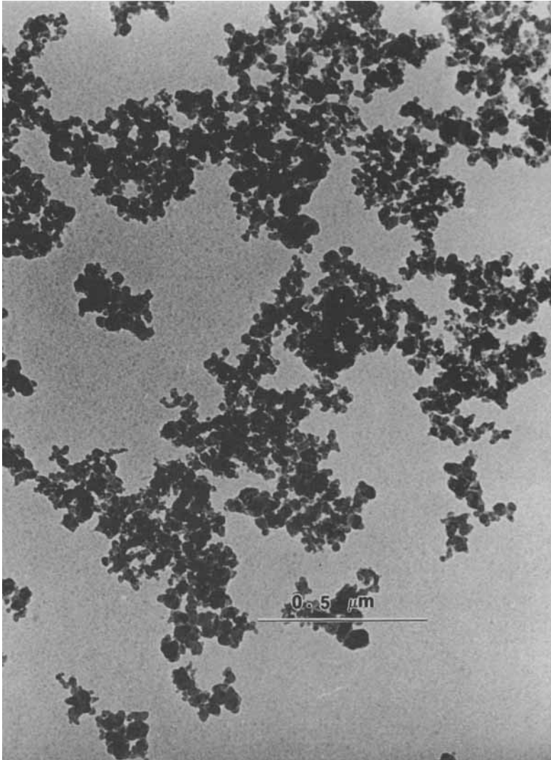
FIGURE 2(b) Smaller carbon black particles demonstrating structure development (electron micrographs courtesy of Ashland Chemical Company).
